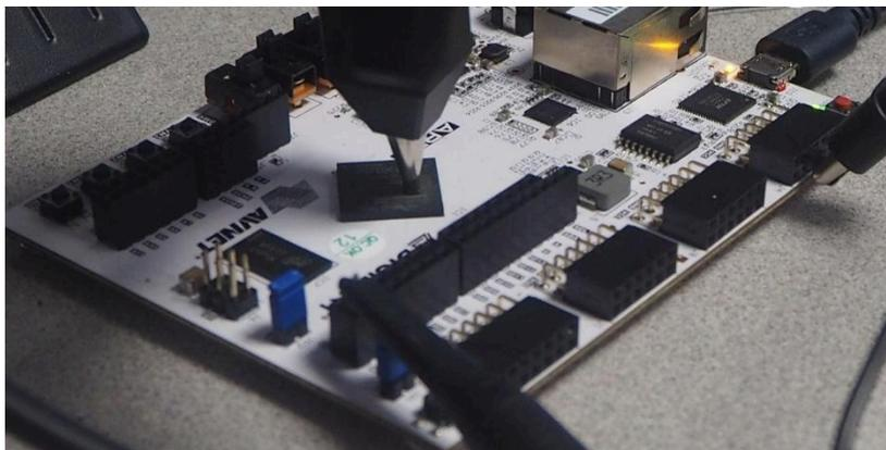
Figure 7: EM probe placed on the main FPGA chip
