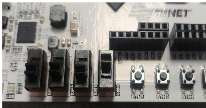
Figure 4: Switches to start the FPGA
