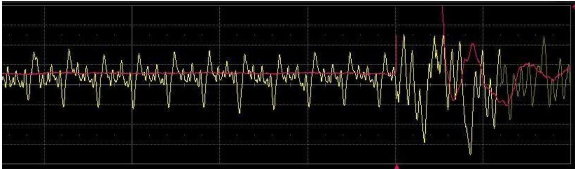
Figure 9: EM waveform with Trigger signal on Oscilloscope
