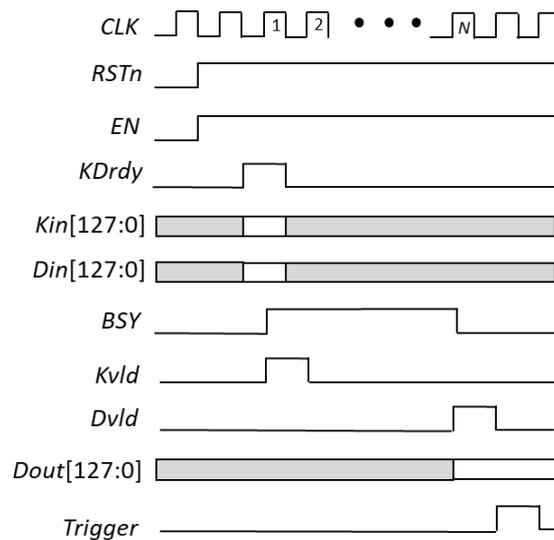
Fig. A2: Interface signals Pattern for a Proper Operation
