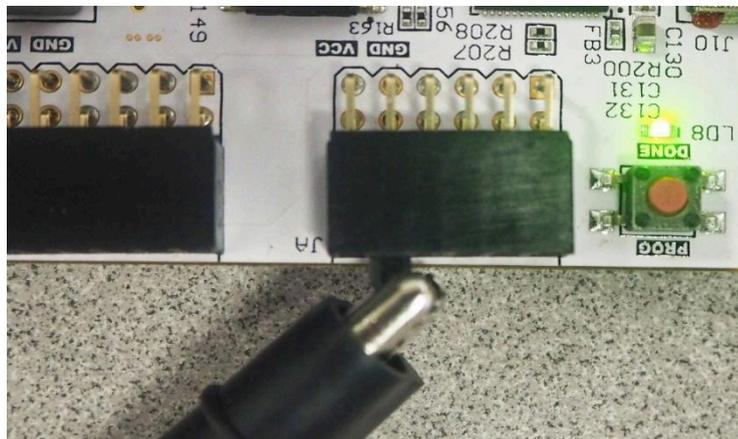
Figure 6: GND connection for your oscilloscope probe
