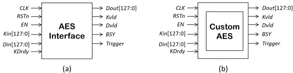
Fig. A1: Interface signals for AES (a) default, and (b) embodying a custom AES
