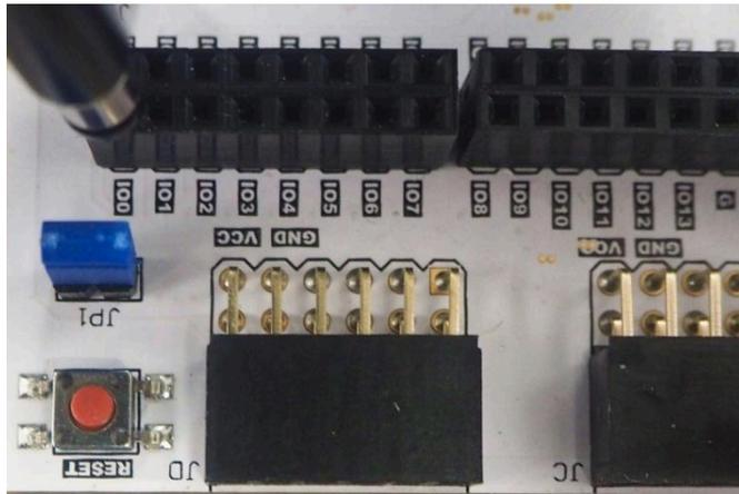
Figure 5: IO0 pin location for oscilloscope probe
